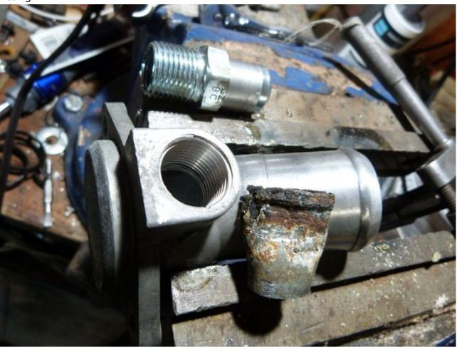
Just unreal how much those top end ports corroded! the bottom end one was only slightly corroded, THANKFULLY.... I was able to file and buff it out to my satisfaction.
