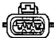
LH Forward Discriminating Sensor Connector
