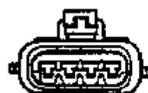
Arming Sensor Connector
